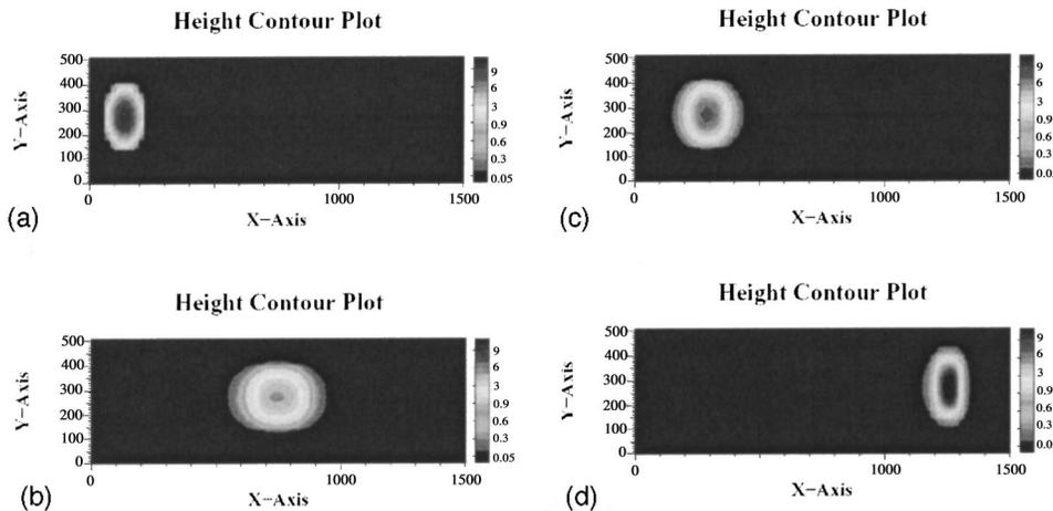
FIG. 3. Granular avalanche down an inclined plane. Contour plots show a paraboloid shape, which can be shown to be a similarity solution of the governing system. The plane makes an angle of  $45^\circ$  until 1000 m, at which point the surface rapidly flattens to become horizontal. The internal friction angle of the flowing mass is  $30^\circ$ , and the bed friction is  $20^\circ$ .
